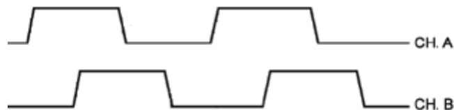
Fig. 4.19: The signals at CH A and CH B outputs of quadrature encoder
