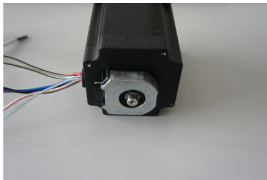
Fig. 3.9: Motor with attached encoder
